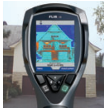
FLIR i3, temperature in 3,600 spots
