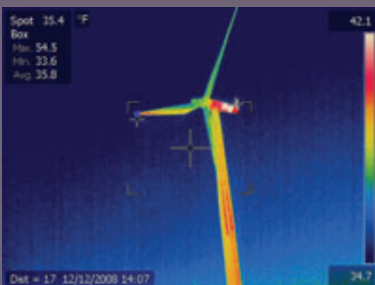
A thermal image of a wind turbine taken from ground level
