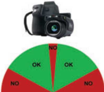
Viewing angle recommended (green) and to be avoided (red) during thermographic inspections.
