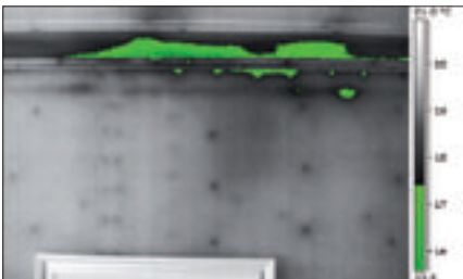
The insulation alarm shows where the areas below or above a set temperature are by making them appear in a different color.
