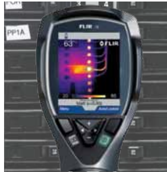
FLIR i3, temperature in 3,600 spots
