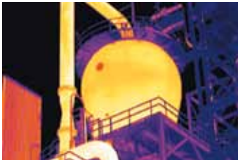
Refractory insulation inspection on a petrochemical reactor
