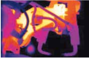
Hot spot in welding robot
